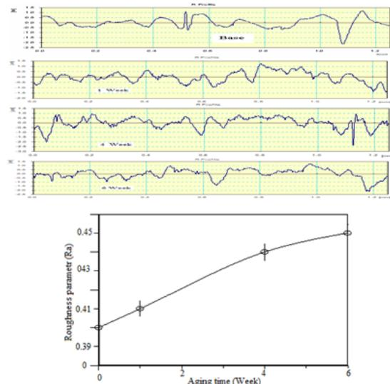
**Figure 3:** (a): Roughness profiles for Ni- Cr based alloy at different time; (b): The roughness parameter Ra for Ni-Cr alloy versus aging time.
