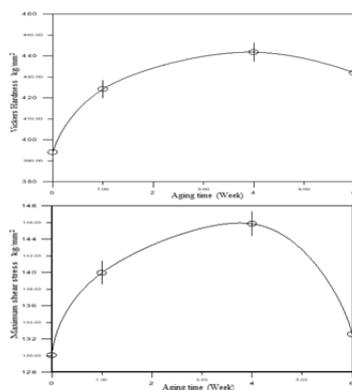
**Figure 2:** Vickers hardness and maximum shear stress of Ni-Cr alloy versus aging time.
