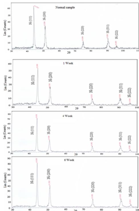
**Figure 1:** X-ray diffraction patterns for Ni- Cr alloy before and after aging in saliva.
