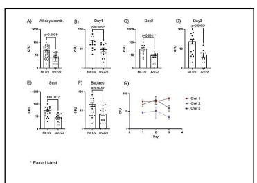
**Figure 2:** Filtered 222 nm excimer lamps reduce bacterial load in hospital waiting area.
